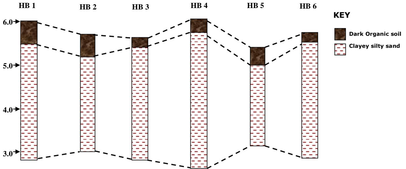
Fig. 2. Soil profile of the construction site (height measured in metres above sea level).
