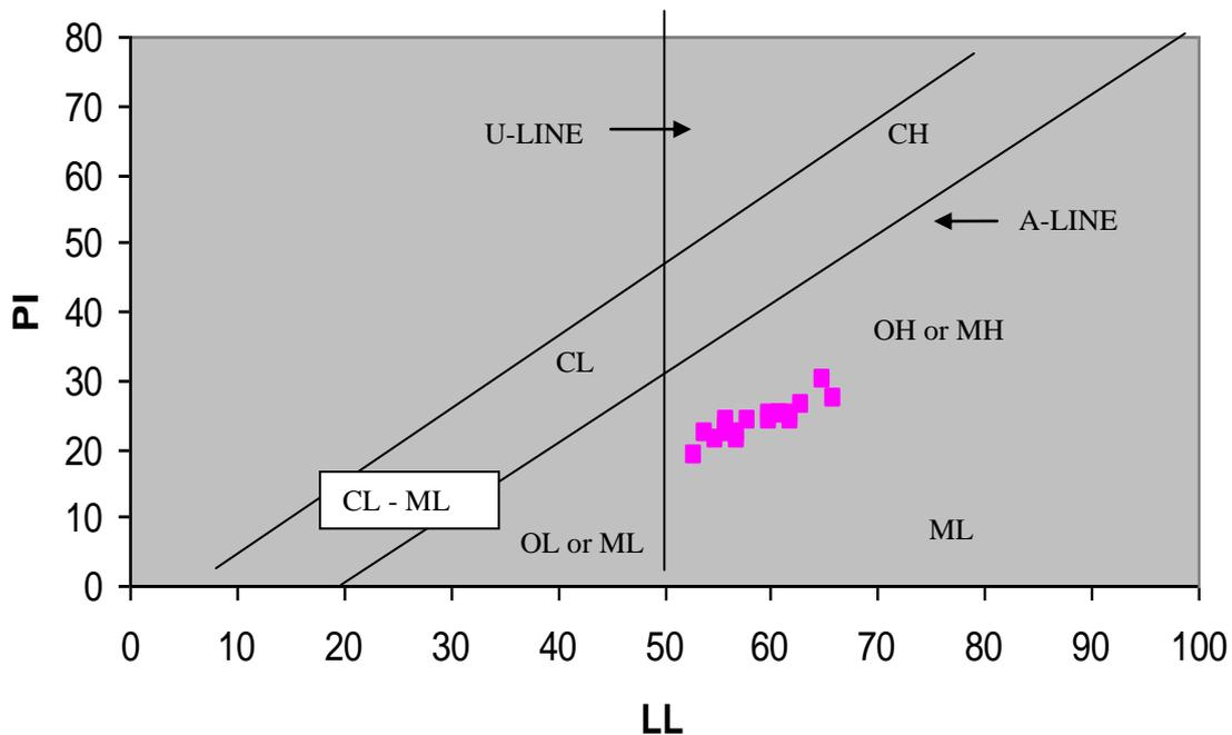
Fig. 5. Mean values of Atterberg limits with depth.
