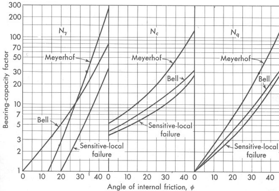
Fig. 3. Bearing capacity factors for general bearing capacity equation.
