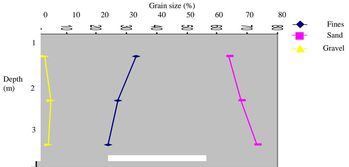
Fig. 4. Mean values of grain size distribution with depth.
