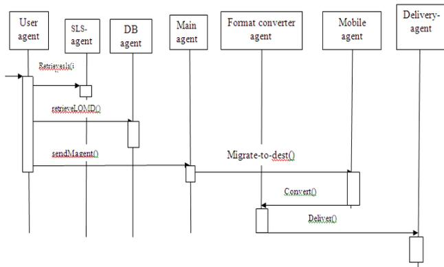
Fig. 2. The sequence Diagram of system agents
