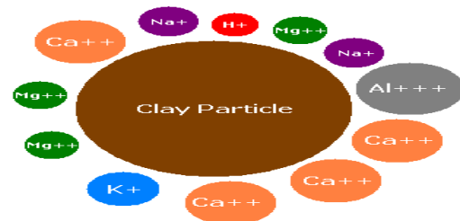
Fig. 1. Clay particle surrounded by different cations.
