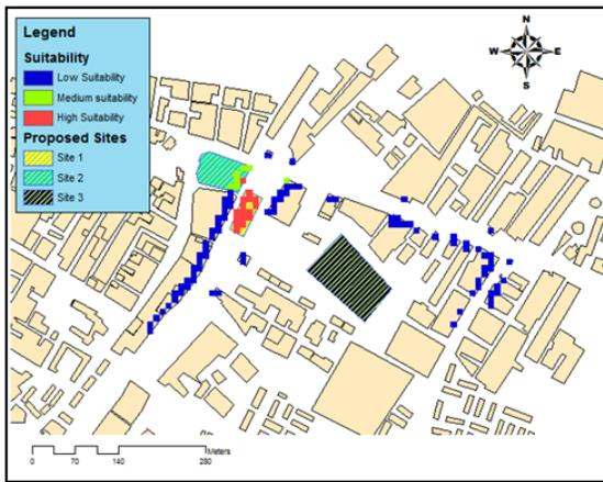
Fig. 11. suitability Map for a wastewater lift station.
