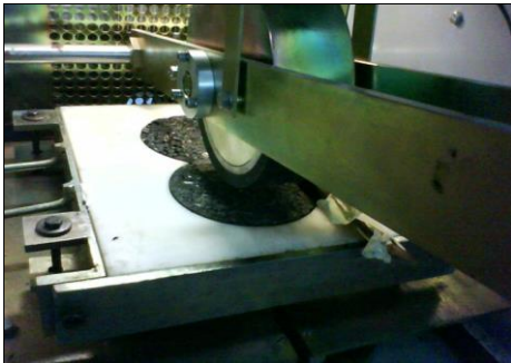
Fig. 4. Wessex wheel tracking test setup
