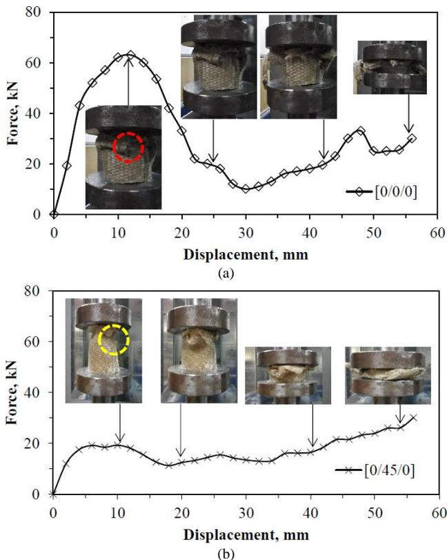
Fig. 5. Effect of fiber orientations on the crushing mechanisms of (a)  $[0^{\circ}/0^{\circ}/0^{\circ}]$  and (b)  $[0^{\circ}/45^{\circ}/0^{\circ}]$ .
