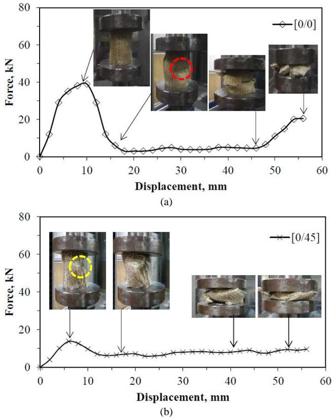
Fig. 4. Effect of fiber orientations on the crushing mechanisms of (a)  $[0^{\circ}/0^{\circ}]$  and (b)  $[0^{\circ}/45^{\circ}]$ .
