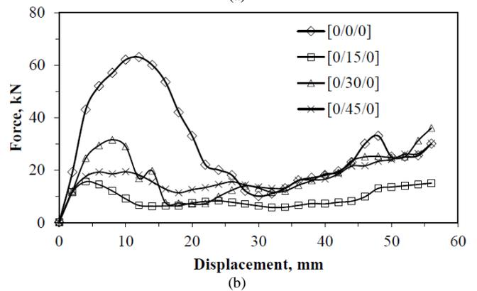
Fig. 3. Force versus displacement curves for (a) two and (b) three layers woven kenaf fiber reinforced composites.
