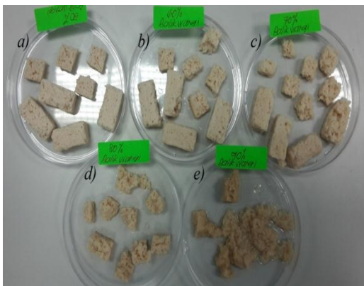
Fig. 2. Scaffolds with percentage of starch; a) 50wt% b) 60wt% c) 70wt% d) 80wt% e) 90wt%
