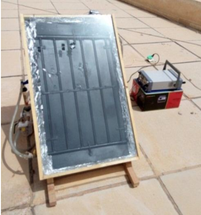
Fig. 1. Flat Plate Solar Collector Experimental Setup
