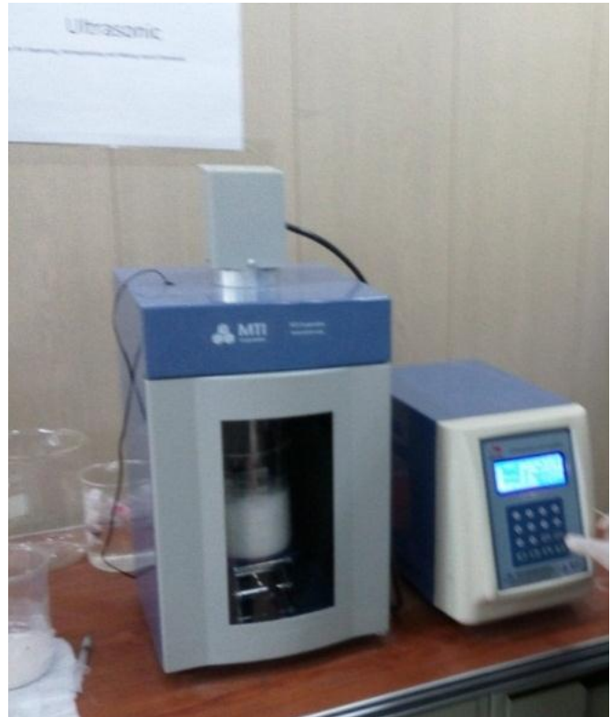
Fig. 5. Ultrasonic Apparatus for Sonication Process of Al_2O_3 -Water Nanofluids
