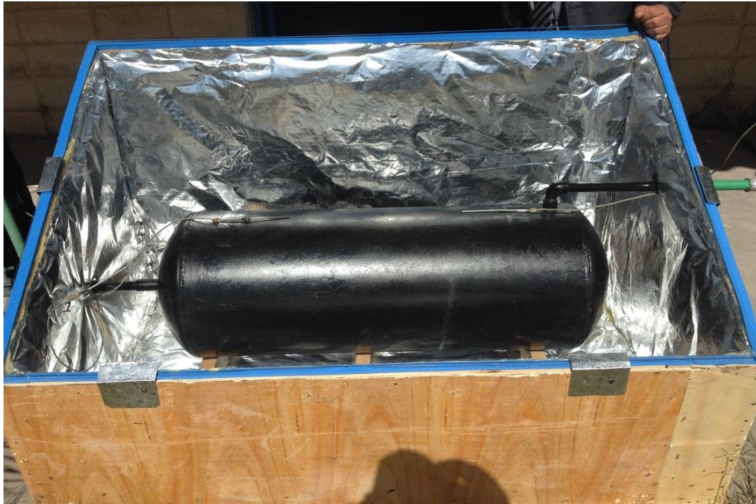
Fig. 1. Assembling of solar water heater
