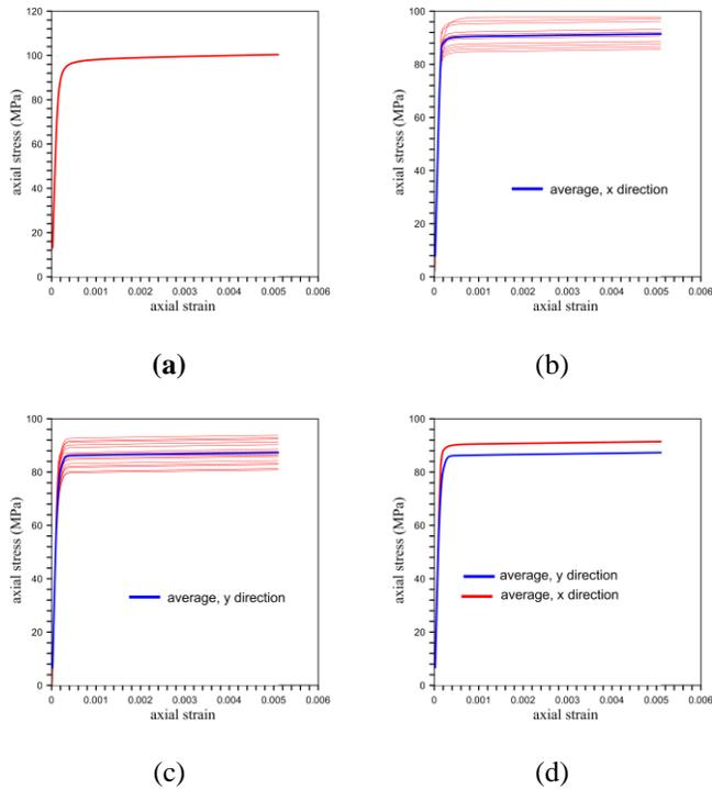
Fig. 4. Apparent stress–strain curves for the 4-phases composite: (a) for the VER ( $p = 1, n = 300$ ) with  $f = 0.7$ , (b) for only one subvolume ( $p = 36, n = 3$ ) stretched in the x direction, (c) y direction, and (d) comparison of average curves in the two directions ( $f = 0.7$ ).
