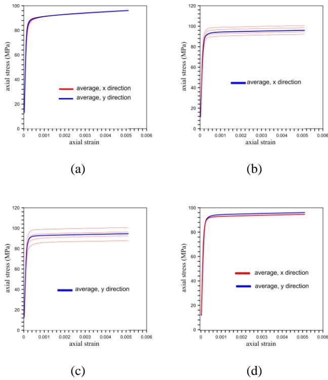
Fig. 3. Apparent stress–strain curves for the 3-phases composite: (a) for the VER ( $p = 1, n = 200$ ) with  $f = 0.7$ , (b) for only one subvolume ( $p = 4, n = 100$ ) stretched in the x direction, (c) y direction, and (d) comparison of average curves in the two directions ( $f = 0.7$ ).
