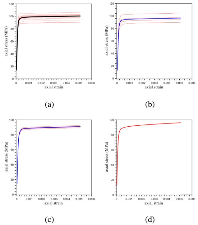
Fig. 5. Examples of apparent stress–strain curves (thin lines) and comparison with the average curve (thick line) for the different configurations of 3-phases material with  $f = 0.7$ : (a)  $n = 24, p = 9$ , (b)  $n = 76, p = 4$ , (c)  $n = 100, p = 4$ , (d)  $n = 200$  and  $p = 1$ .
