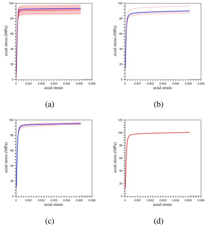
Fig. 6. Examples of apparent stress–strain curves (thin lines) and comparison with the average curve (thick line) for the different configurations of 4-phases material with  $f = 0.7$ : (a)  $n = 3, p = 36$ , (b)  $n = 99, p = 4$ , (c)  $n = 150, p = 4$ , (d)  $n = 300$  and  $p = 1$ .
