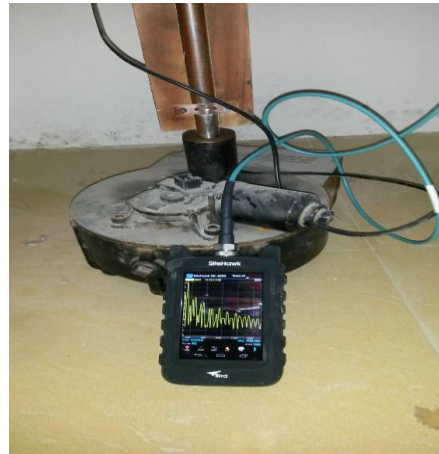
Fig. 18. VSWR Measurement setup
